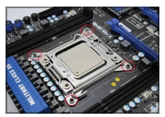
Ensure the CPU is fitted correctly into the Motherboard, then apply paste to the CPU to the top as required. Only a small amount is needed to produce a thin layer, then smooth it down with a flat plastic card or spatula making sure you clean up any excess with a tissue or an alcohol wipe.
