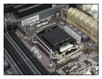
Ensure the CPU is fitted correctly into the Motherboard, then apply paste to the CPU to the top as required. Only a small amount is needed to produce a thin layer, then smooth it down with a flat plastic card or spatula making sure you clean up any excess with a tissue or an alcohol wipe.
