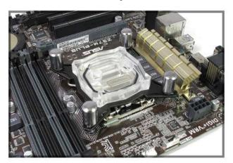
Take a thumb screw, and thread it onto each mounting screw as above, as far down as you can just before the spring starts to make tension. Repeat this for the others. Once all four of the thumb screws are in place, you can start to tighten them down opposites at opposite corners so that the tension is evenly applied. Tighten them until the thumb screw stops.
