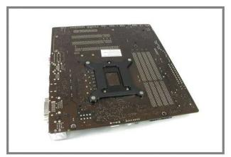
Take four of the washers you have received in your mounting pack and place them over the four Intel mounting lugs as shown below. From the same mounting pack, find the mounting screws, and thread them into the 115X backplate to secure it in place, making sure the washer is separating the mounting screw from the Motherboard.
