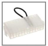
Plug this tool into your Powersupply, it will allow you to start the PSU without the Motherboard being switched on.
